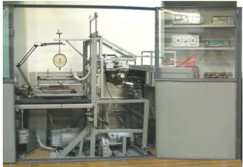
Pic. 4. Current collectors and conducting wire interaction simulating bench for metro, third rail and monorail systems
